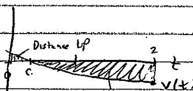
A] Total distance =  $\int_0^2 |v(t)| dt = \int_0^2 v(t) dt = 0.454 \text{ m}$
